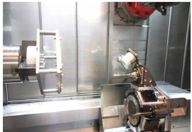
where a partial die could be used on a turret as a kinematic supporting tool which can follow the forming tool somewhat like a potter, using its hands to form a clay pot. This will allow for increased control of accuracy and thickness.
